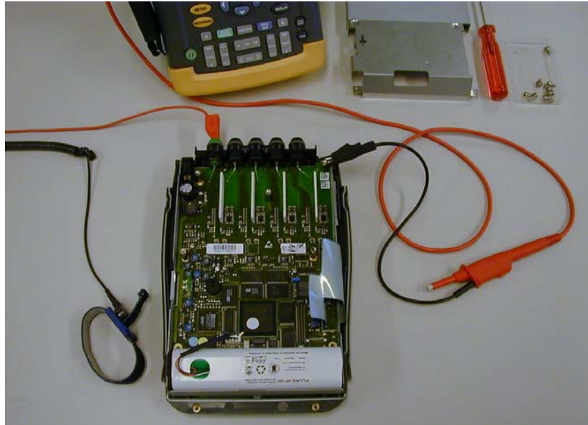
Figure 7-1. Operative Analyzer, Measuring on Top Side
